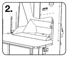
To extend or retract the panel, lift the handle on either side of the swarf collector and push or pull in the direction required.
