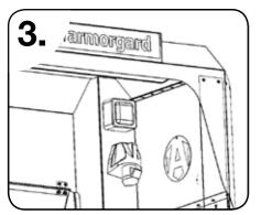
Inside the CuttingStation a switch is located in the top right corner for operating the work light.
