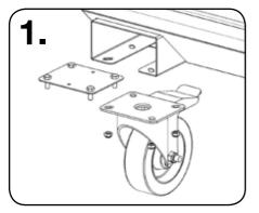
Fix castors using the castor plates, wheels, and nylocks provided. Slide the castor plate into the forklift skid and drop the welded on bolts through the pre-drilled holes in the skid.
