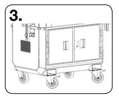
We recommend you position the two swivel-braked castors so they are at the front of the unit, and the two swivel castors at the rear.
