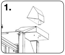
Position the swarf collector in the centre hole at the back of the work bench, and fix in place using the 2x M6 bolts provided.
