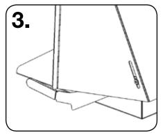
When the back panel is extended, the handles on either side drop down to lock it in position.
