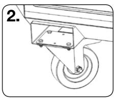
Locate the castor wheel on the bolts of the castor plate, and then tighten all nylocks, ensuring they are fully on the thread of the bolt.
