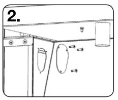
The plate can be removed and refixed with the three screws.
