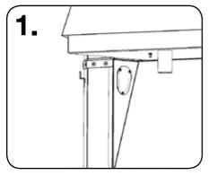
At the rear of the CuttingStation is a blanking plate that can be removed to allow cables, extraction hoses etc to be fed into the cabinet beneath the work surface
