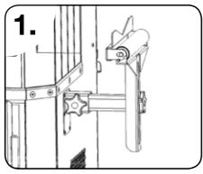
The two locking screws on the support arm can be loosened to allow the support arm to slide in and out, and up and down.
