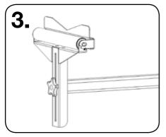
The support arm head can be turned 90 degrees for a v-shaped support to hold round materials. Note that in this position the flat surface can also be used as a stop for efficient cutting.
